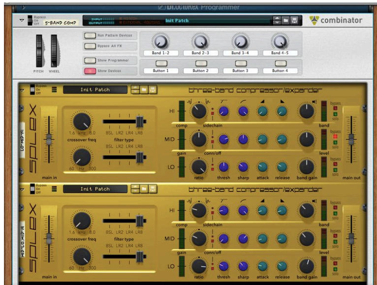
Figure 5: Front panel settings for five-band compressor
