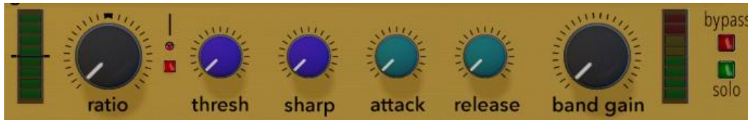
Figure 4: Compression section for a single band
